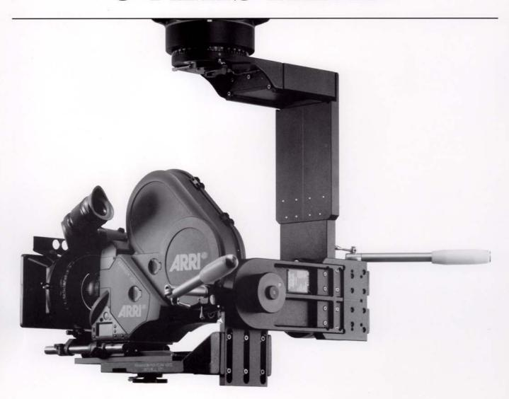
The Ronford-Baker Fluid 7 3 AXIS Head is designed for use with either film or video cameras up to 25KG. The three fluid units are controlled through seven stages. All three axis are continuous through 360 degrees. The head can be adjusted to the cameras centre of gravity. This unit, with the addition of one angle bracket, is built up from standard F7 head components.
