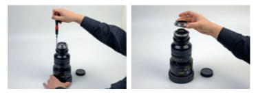
3. Remove the torx screws of the silver EF adapter ring and place the ring and the screws on one side.
