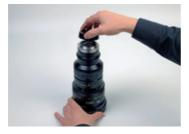
2. Remove the torx screws of the silver EF mount with a T6 torque wrench and place the mount and the screws on one side. The size of the black inner ring is securely fastened to the EF mount at the factory.
