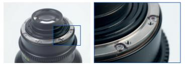
6. Now place the PL mount on the lens in such a way that the groove on the underside of the PL mount fits over the silver screw on the lens barrel. Tighten the torx screws with the T6 torque wrench using a torque of 0.4 Nm.
