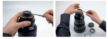
13. Please lign up the EF mount with the EF adapter that the four screw holes are lying upon each other.
