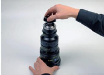
2. Remove the torx screws of the silver EF mount with a T6 torx wrench and place the mount and the screws on one side. The size of the black inner ring is securely fastened to the EF mount at the factory.
