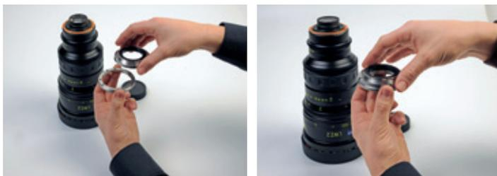
14. Now place them on the lens in such a way that the groove on the adapter ring is facing to the index ring on the lens barrel. Tighten the screws of the EF adapter ring and then the screws of the EF mount using a torque of 0.4 Nm. Please note the different lengths of the torx screws to tighten the different LWZ.2 mounts:
