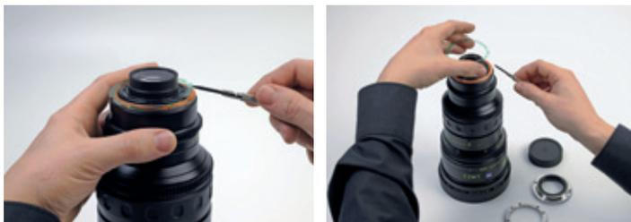
13. Please align up the EF mount with the EF adapter that the four screw holes are lying upon each other.
