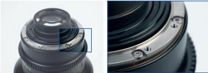
6. Now place the PL mount on the lens in such a way that the groove on the underside of the PL mount fits over the silver screw on the lens barrel. Tighten the torx screws with the T6 torque wrench using a torque of 0.4 Nm.
